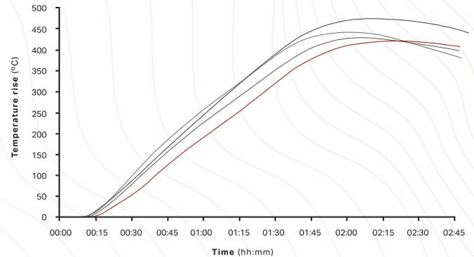
In such conditions, a temperature increase of 100°C inside the SUM Fire Guard® cover is reached after up to **30 minutes!**
