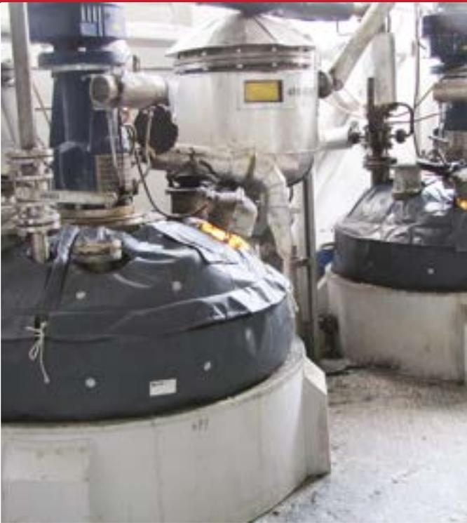
**SUM Chemical Guard®** covers significantly improve the work of maintenance teams offering instant access to, for example, flange gasket leaks, allow quick identification of the leak, its repair and re-installation of insulation. SUM covers do not undergo any degradation during such operations and allows for performing of routine inspections and maintenance work without the participation of outside insulators.
